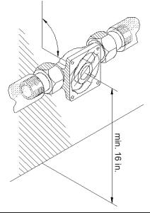
Until final assembly the adhesive label which serves to protect the sealing surface is to remain on the housing flange (remove it immediately before final assembly).
