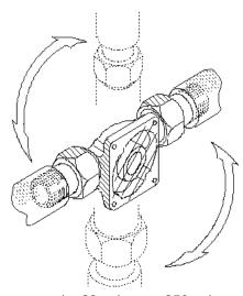
Inlet pressure min. 29 psi, max. 250 psi. Operating medium: potable water
