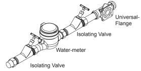
Observe the minimum distance between floor and centreline of the pipe installation (16 in.).
