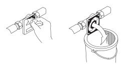
Before attaching the filter to the flange, rinse the flange with about 1/2 gallons of water into a bucket.
