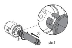
With the other side of the tool, remove the backflow preventer from the housing. Insert the tool again and turn the RV out counterclockwise (pic 4).
